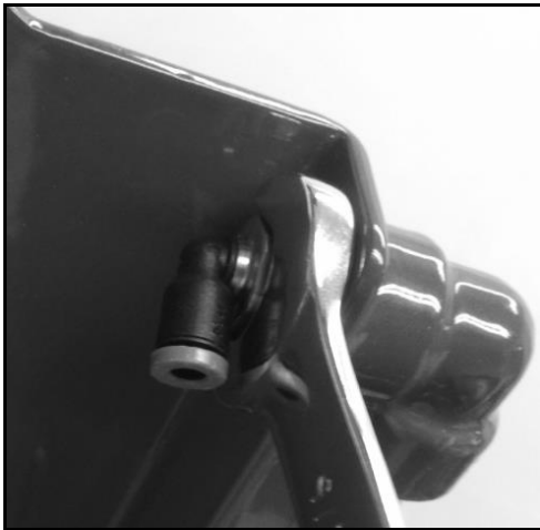
Threaded elbow fitting
